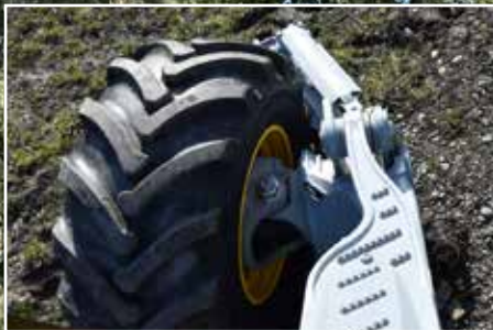
Mountain stabilizers automatically not within operating range
