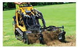
BUILT TO PERFORM. Get more out of each day with a tipping capacity of 2643 lb (1198.8 kg) and rated operating capacity of 925 lb (419.6 kg) while reaching to maximum hinge pin height at 84.5" (214.6 cm).
